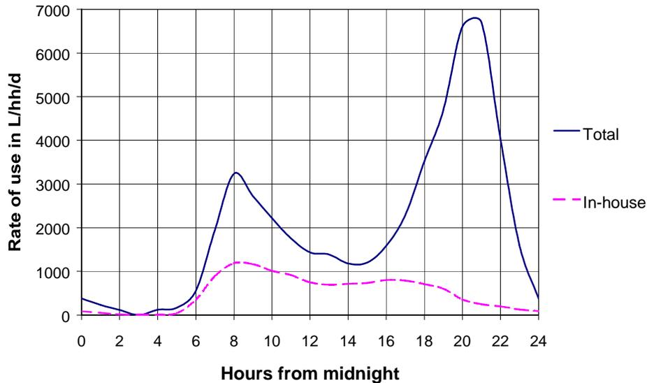
Figure 2: Design curve of diurnal variability in water supply
