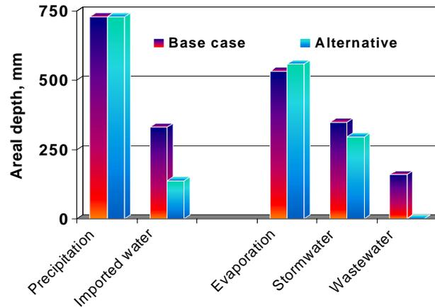
Figure 4: Change in water inputs and outputs
