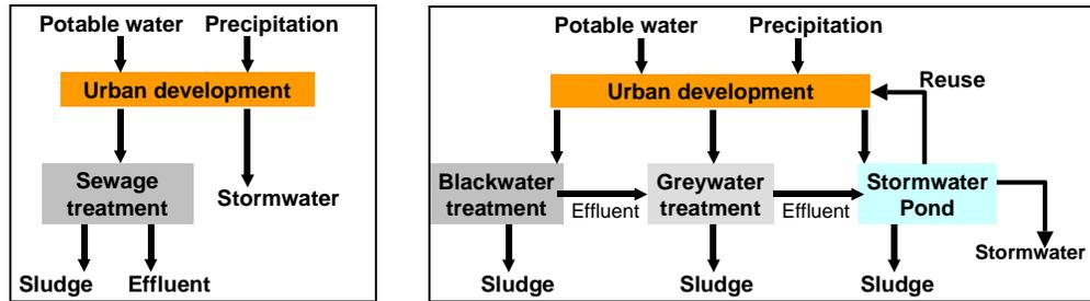
Figure 3: Base case and decentralised stormwater and wastewater utilisation system
