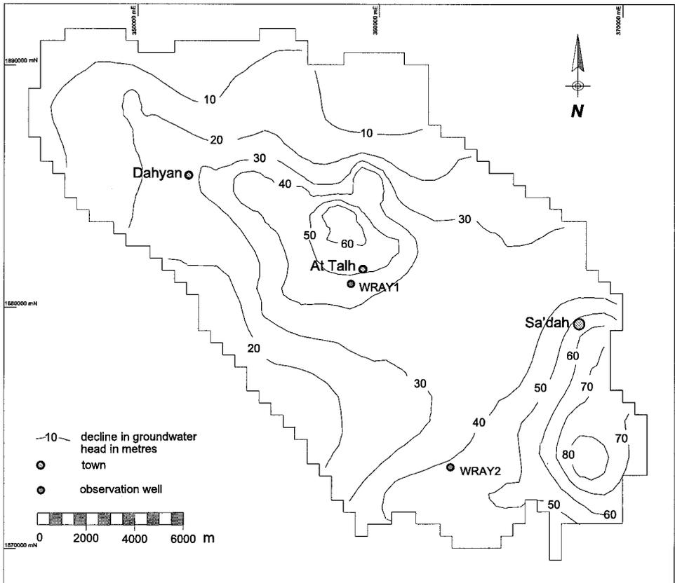
**Figure 6.** Decline in groundwater levels from 1978 to 1992 according to the calibrated groundwater model.
