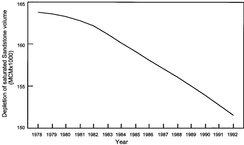
**Figure 7.** Diminishing volume of saturated sandstone as calculated by the calibrated groundwater model.
