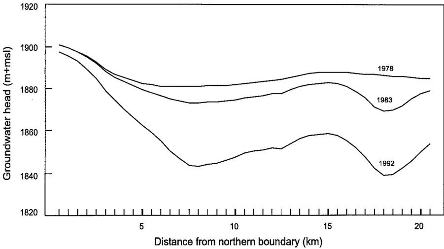
Figure 5. Fall of piezometric levels along section A-A of Figure 2.
