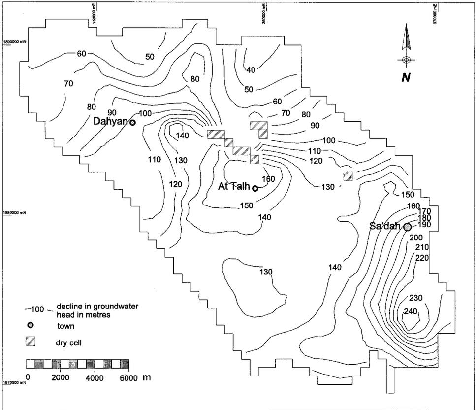
**Figure 8.** Decline in groundwater levels 1978–2020 under present conditions according to the calibrated groundwater model.
