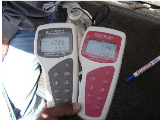
Figure 1-3 Measurement of EC and PH in the field directly after collecting water sample
