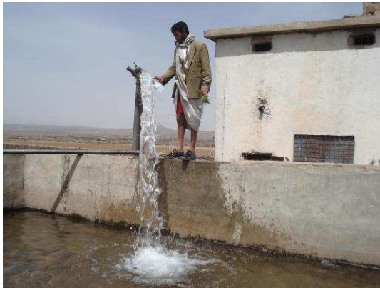
Figure 1-2 Collection of a water quality sample from the pump outlet
