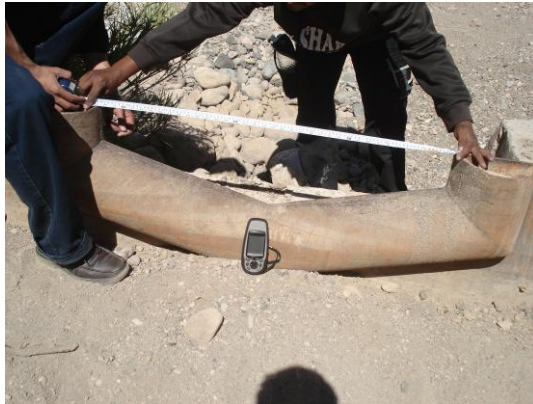
Figure 6-104 V-Notch during field measurements
