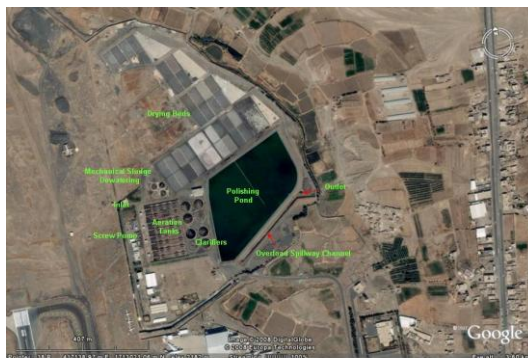
Figure 6-111 Google Earth picture showing the general layout of the Sana'a Wastewater Treatment Plant
