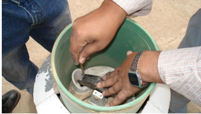
Figure 2-22 Regular maintenance for the rainfall station is performed by removing the dust from the inside parts of the station
