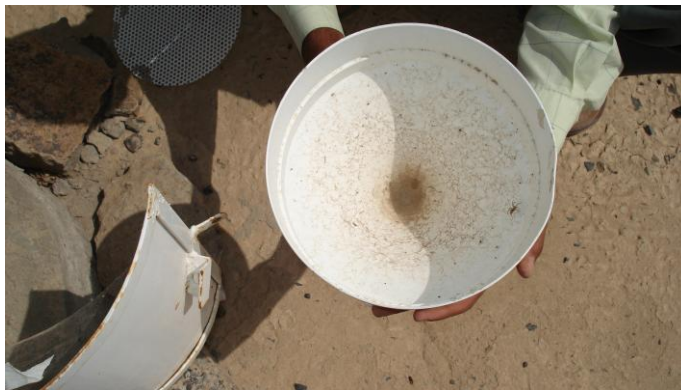
Figure 2-17 Sometimes dusts or insects houses blocks the funnel opening
