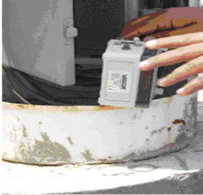
Figure 2-14 Rainfall station data logger (this system is used in all stations)
