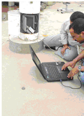
Figure 2-15 Applied procedure for collecting digital data from rainfall station data logger
