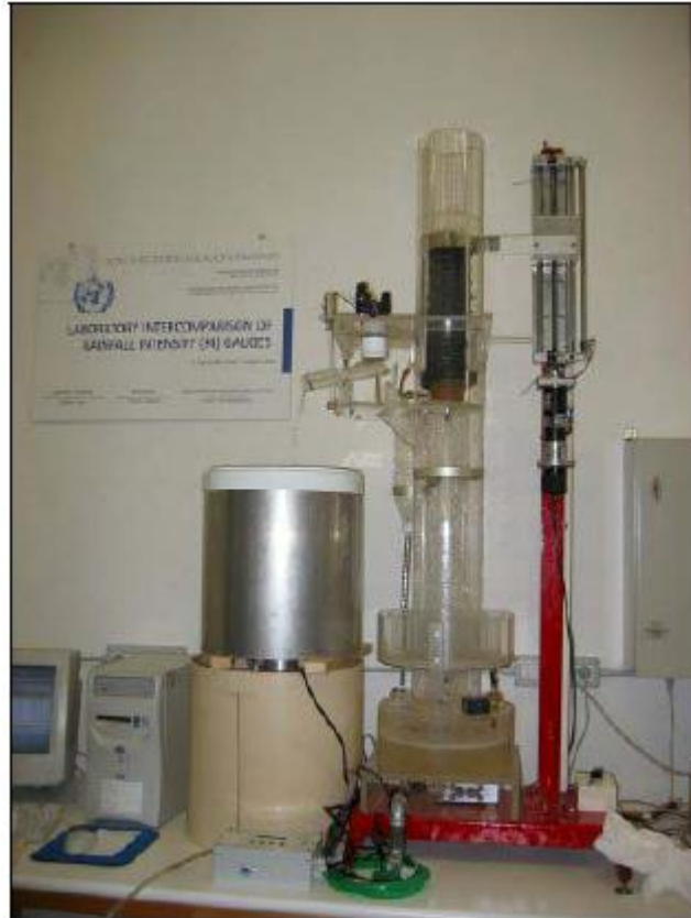
Figure 1-1 Inter-comparison laboratory experiment for a tipping-bucket rainfall
