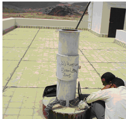
Figure 2-10 Shahek rainfall station on the roof of Shahek school
