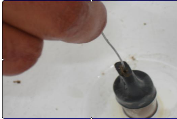
Figure 2-19 Cleaning the nozzle opening at the funnel bottom side
