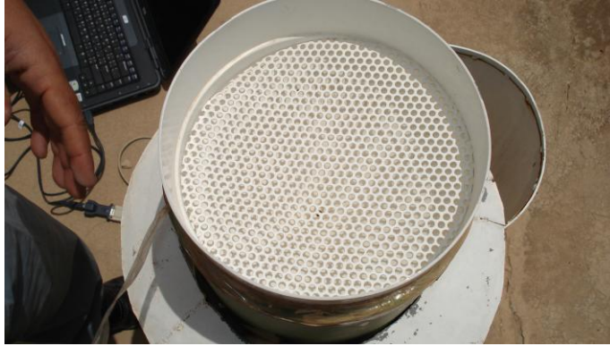
Figure 2-16 Top view of water bucket collector showing the screen
