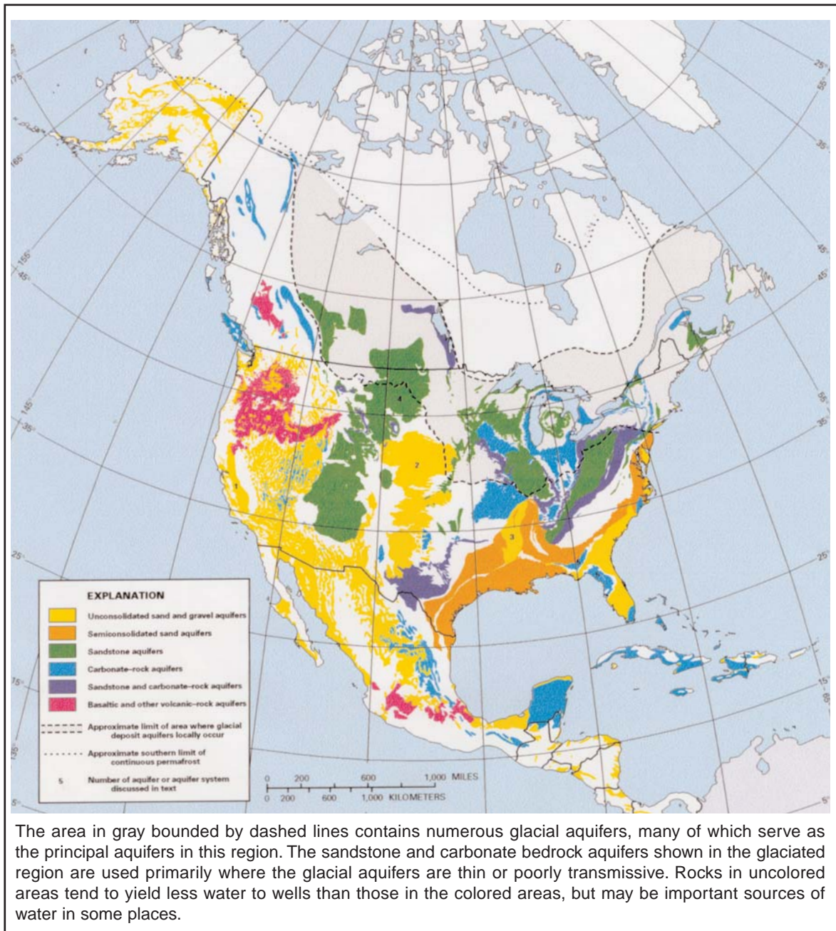
Figure 5.3.3.1 Map showing uppermost principal aquifers in North America (Modified from Miller, 1998; Heath, 1988; Back et al., 1988 and North American Geologic Map Committee, 1965)
