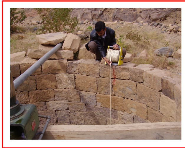
Monitoring wells water level by using Electric Sounder
