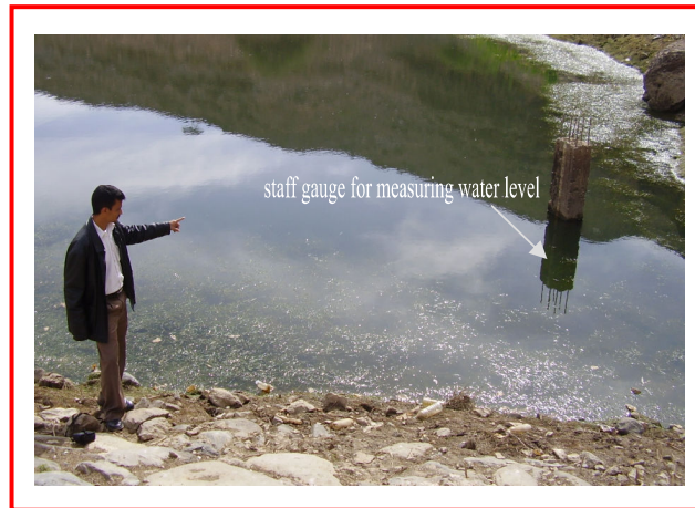
Photo shows the monitoring of water level in the Mekhtan dam (staff gauge)
