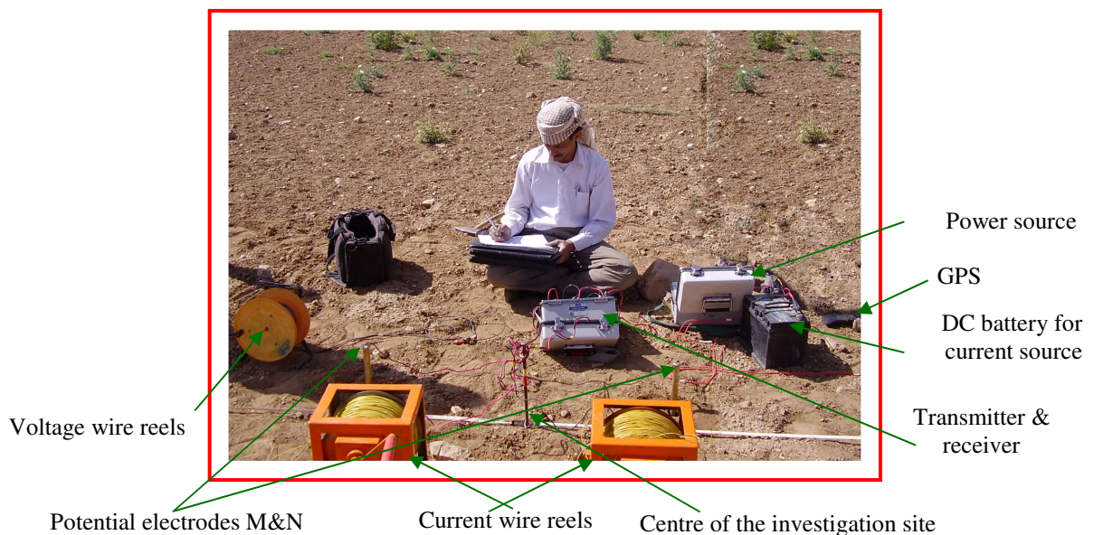
Figure 4.3 Field instruments, IRIS instrument SYSCAL R2 resistivity meter and the other tools.
