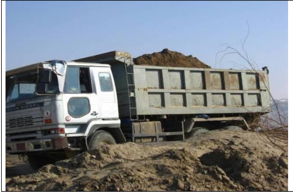
Uncovered Hauling of Dirt Observed During Field Visit
