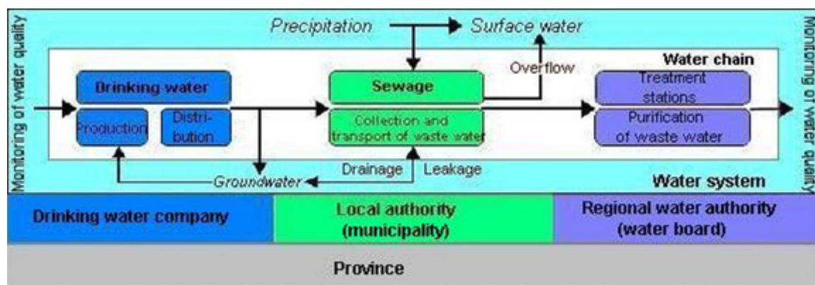
Figure 2: The water system and water chain in Dutch water and environmental legislation
