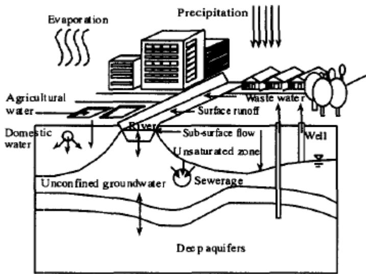
Figure 4: Schematic impression of hydrological water cycle in urban areas (Imbe *et al.*, 1997)
