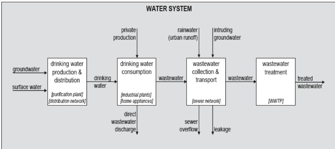
**Figure 3: Schematic representation of the urban water chain (Bots, 2008)**
