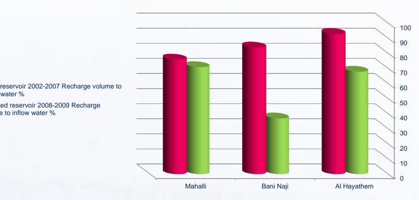
hecks dams show highest efficiency of recharge llowed by smaller gravity dams. Check dams rove to be an excellent vehicle to engage local ommunities in practical action for water esources conservation.
