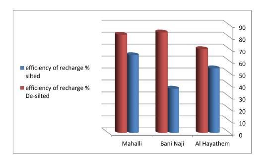
Checks dams show highest efficiency of recharge followed by smaller gravity dams. Check dams prove to be an excellent vehicle to engage local communities in practical action for water resources conservation.
