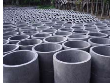
Concrete rings for lining open wells in India
