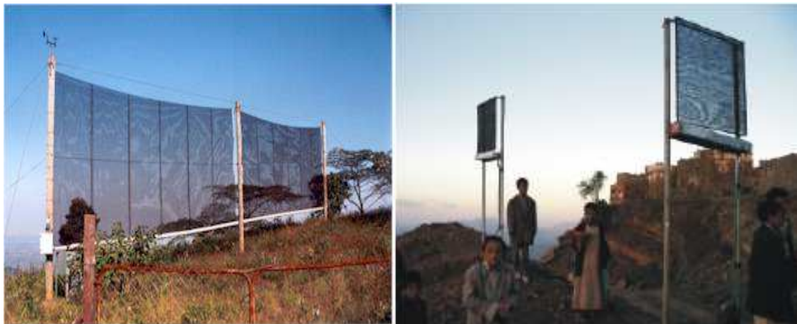
Plate 1 Big (3x2) m 2 and small (1x1) m 2 fog collectors in Hajjah area in Yemen (Authors)
