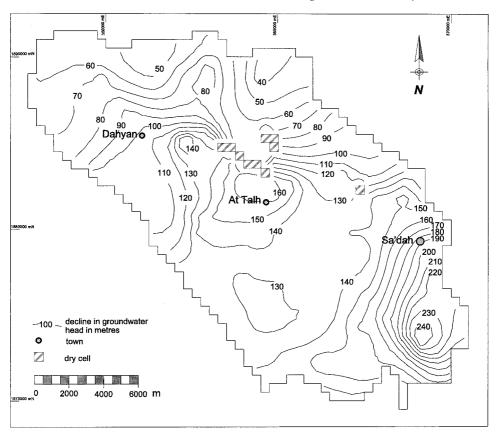
Figure 8. Decline in groundwater levels 1978–2020 under present conditions according to the calibrated groundwater model.
