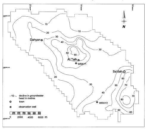
Figure 6. Decline in groundwater levels from 1978 to 1992 according to the calibrated groundwater model.
