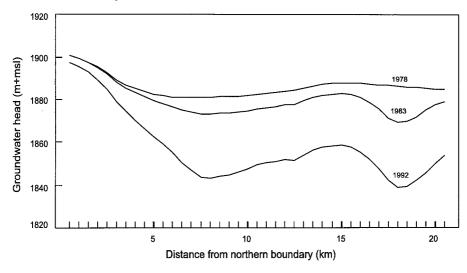
Figure 5. Fall of piezometric levels along section A-A of Figure 2.
