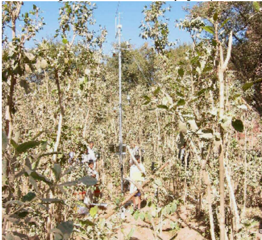
Figure 15: Micrometeorological Modified Bowen Ratio station (MBR station) after installation at Al-Qabil on 10th Feb. 2005 (Photo: W. Kaspari)
