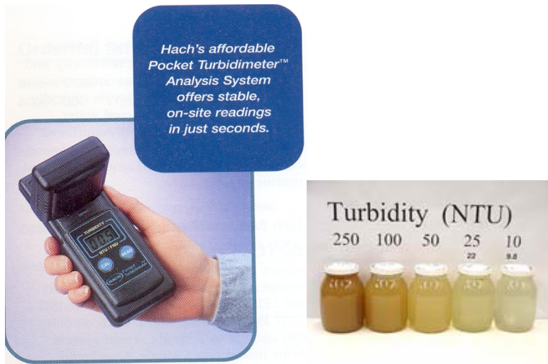
Figure 2-8: Turbid meter and example samples.
