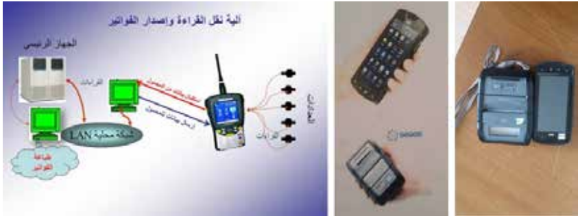
Figure 2 Handheld personal digital assistant system including handheld printer
