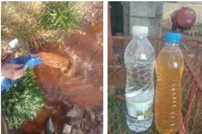
Figure 19 Untreated source water with high iron concentration and treated water
