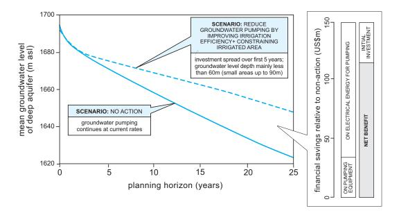
Figure 4: Output of management scenario modelling for the Silao-Romita aquifer system using current MODFLOW numerical aquifer model integrated with economic data for selected agro-production regimes
