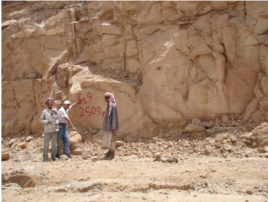
Photo 3-27 Preparation of rock sample from Medj-zir Formation - Lahima member
